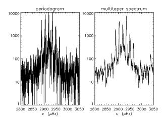
increasing the number of tapers a multitaper spectrum can be made as smooth as desired, but as a trade-off the narrowest modes are then eliminated. The useful number of tapers is on the order of five.
